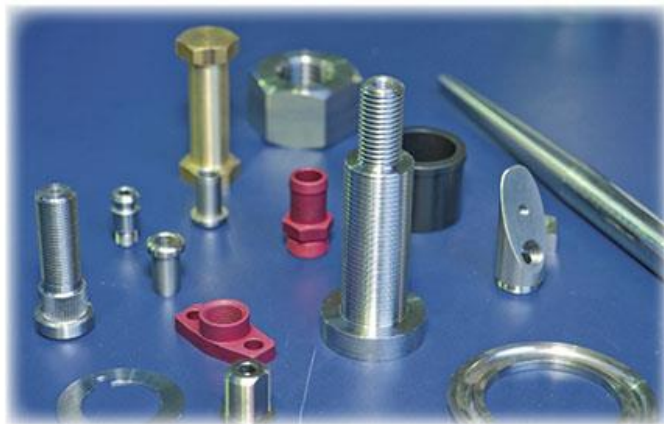
New technology ... components machined using a multi-axis CNC lathe
