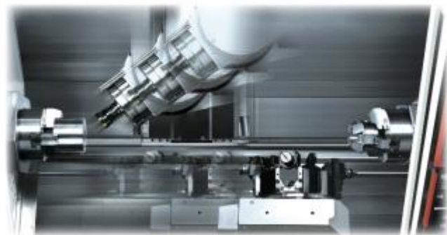
Machining component using B-Axis and lower turret on sub-spindle
