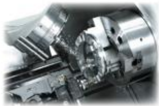
(2nd spindle) Machining component using B-Axis and lower turret on sub-spindle
