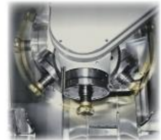
(overall view) Utilising B-Axis and lower turret on main spindle
