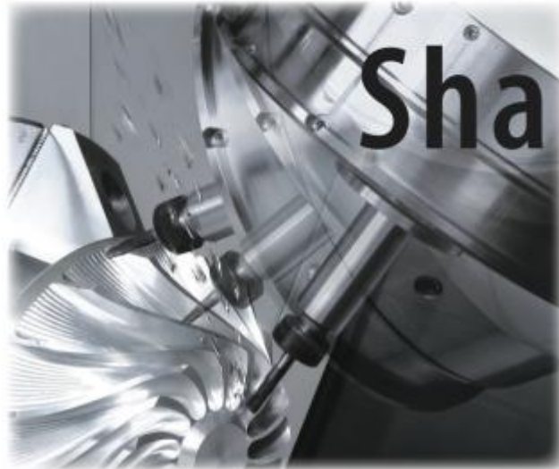
(C-Axis and B-Axis) Utilising B-Axis and C-Axis for complex parts
